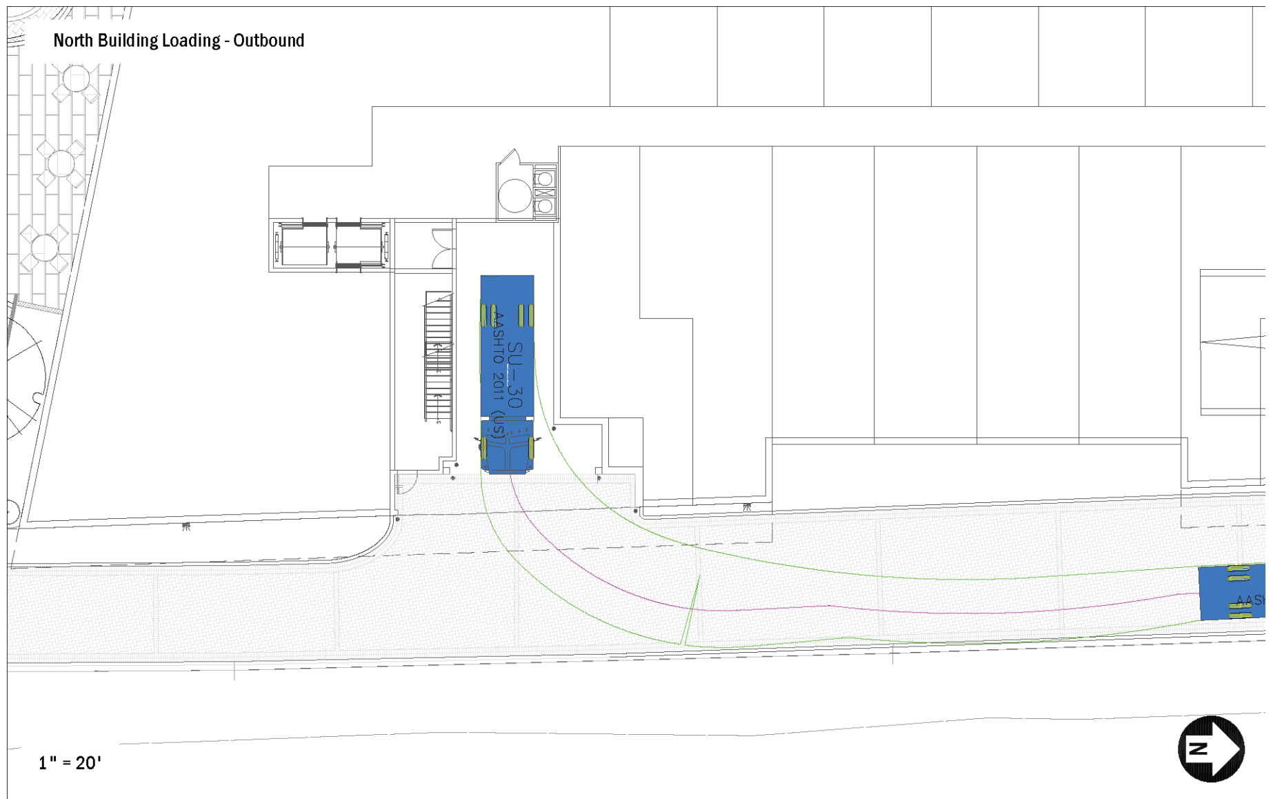
Figure 12: Truck Turning Maneuver (North Building, Outbound)
