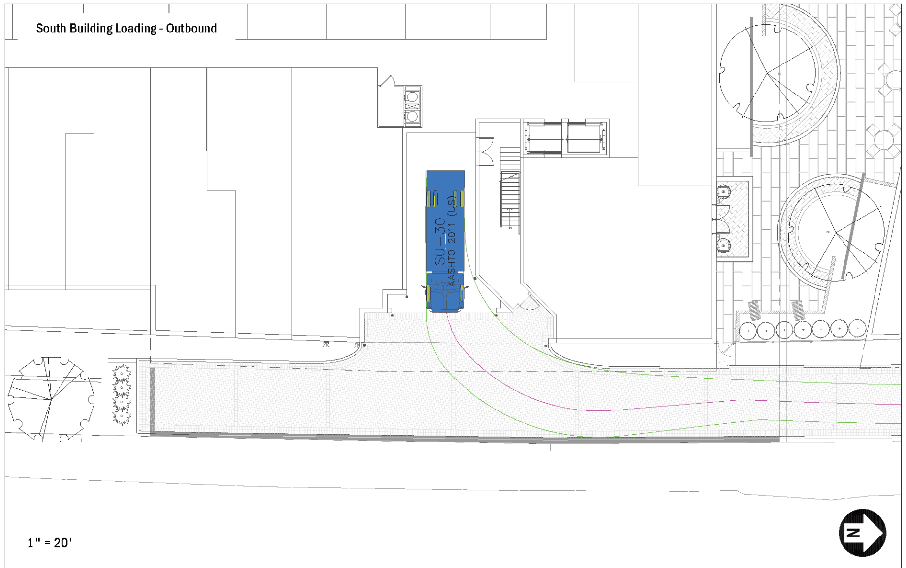
Figure 14: Truck Turning Maneuver (South Building, Outbound)
