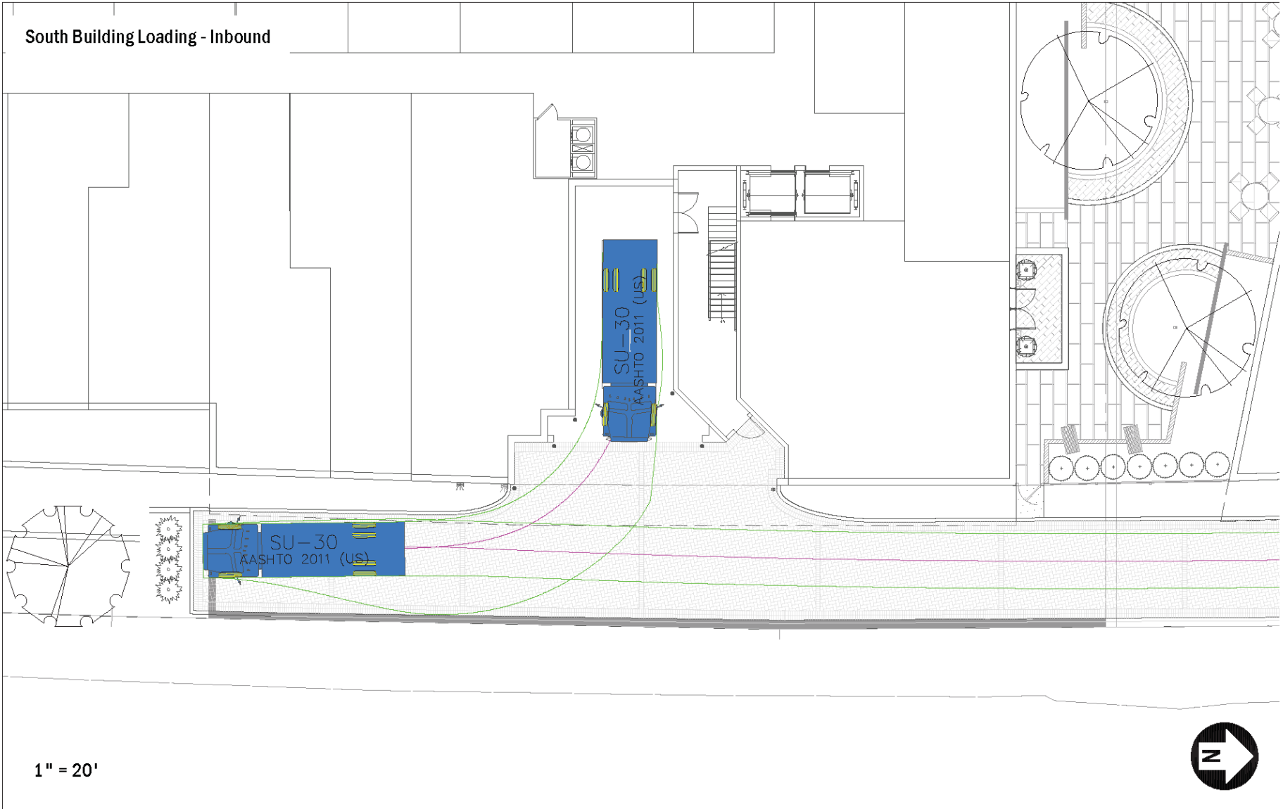
Figure 13: Truck Turning Maneuver (South Building, Inbound)
